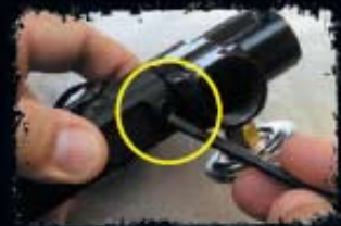
Remove LPR Retaining Allen
