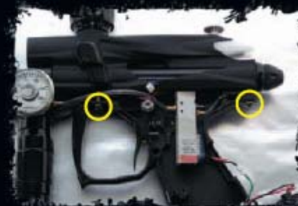
Remove Frame Mounting Screws
